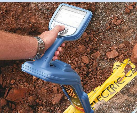
Accurately locating and marking buried assets ensures minimum downtime during repair or maintenance activities. It also prevents damage, which can be costly for both excavator and utility owner.
