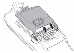
Figure 4.6 installing a new battery pack
