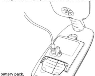
Figure 4.12 Charging the locator Li-ion battery pack
