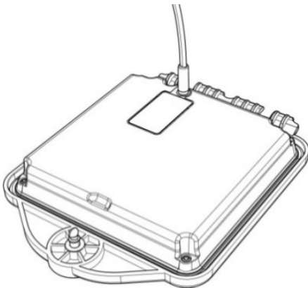
Figure 4.13 Charging the transmitter Li-Ion battery pack
