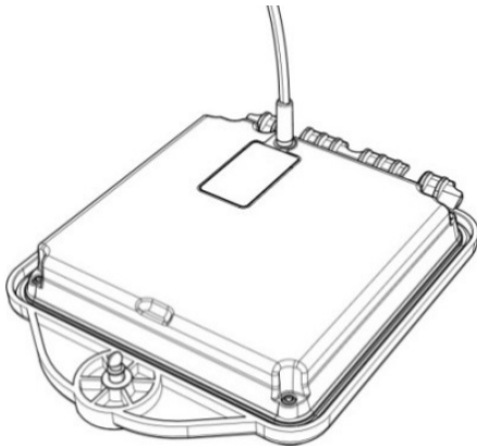
Figure 4.13 Charging the transmitter Li-Ion battery pack
