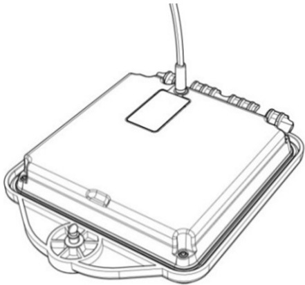
Figure 4.8 Charging the transmitter Li-Ion battery pack
