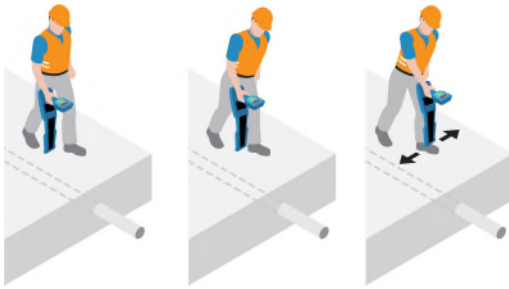
Figure 5.6: Pinpointing a target line
