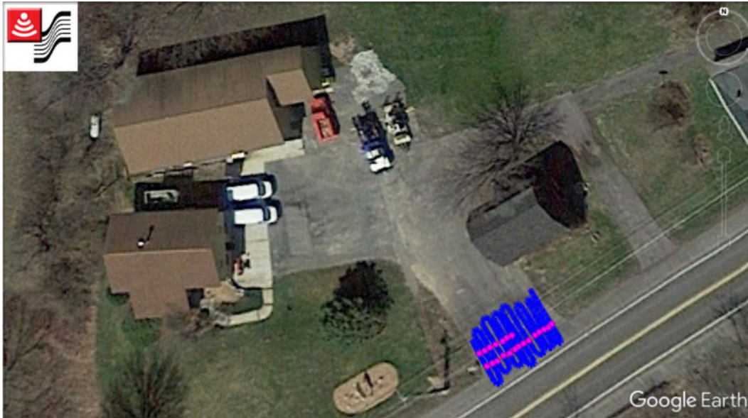
Figure 11-6: Path travelled with Interpretations, collected using an External GPS
