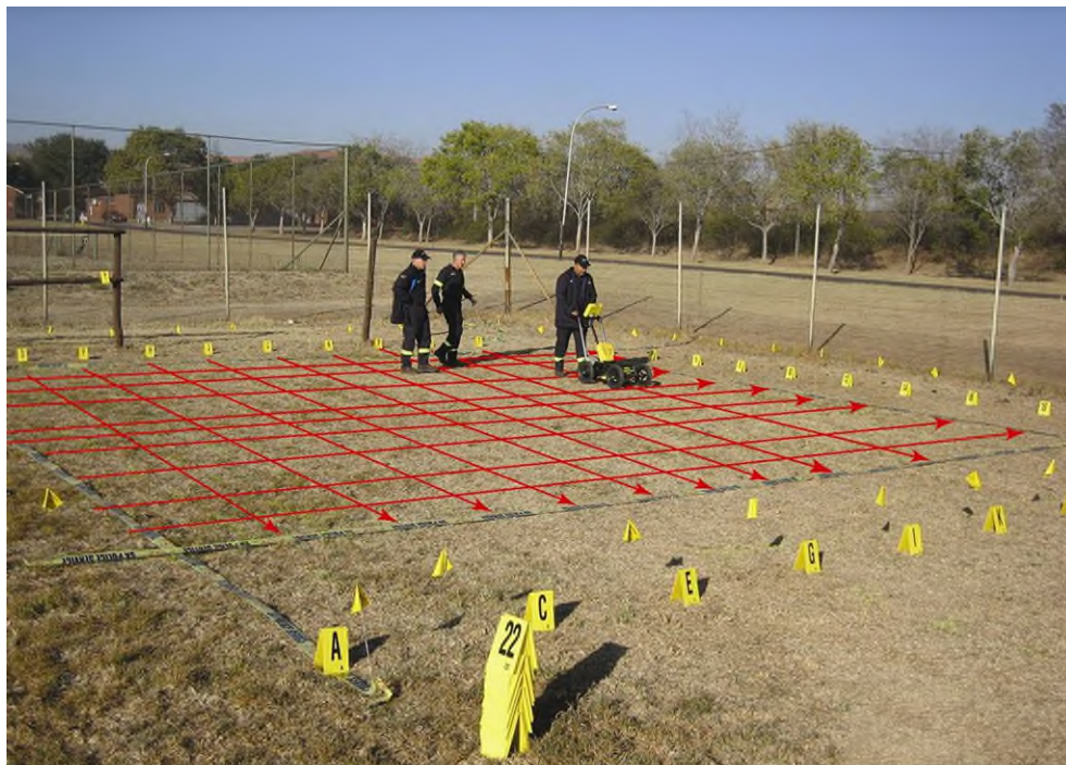
Figure 7-7: Example of a grid survey. The red lines are superimposed just to illustrate the concept.
