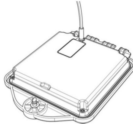
Figure 4.13 Charging the transmitter Li-Ion battery pack
