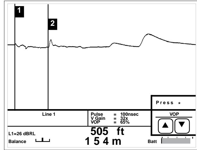
An intermittent open at the 2nd cursor is trapped by the Intermittent Fault Detection (IFD) Mode.
