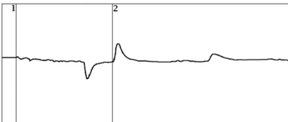
The distance between the two cursors is the distance from the TDR to the end of the lateral.
