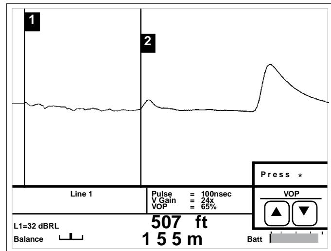
The middle reflection at the 2nd cursor is a ONE SIDE PARTIAL OPEN followed by a COMPLETE OPEN (end of the cable). The more severe the fault, the larger the reflection will be.
