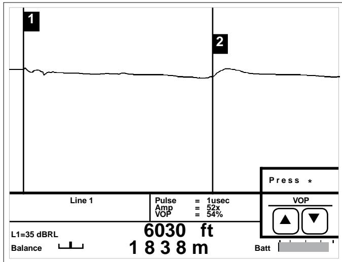
An open at 6030 feet on twisted pair cable. Increasing the pulse width and vertical gain is necessary to see a distant fault.
