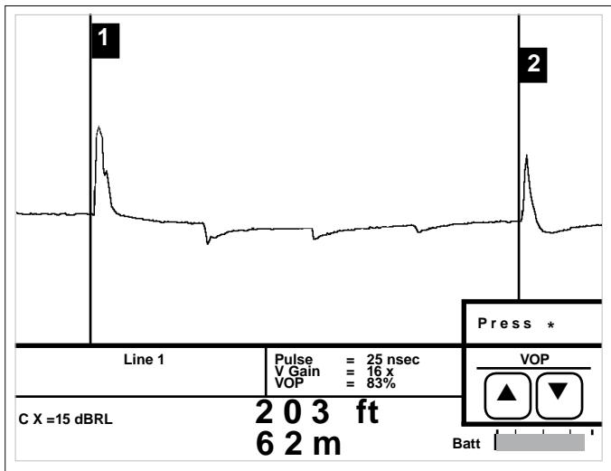
Coaxial taps (both indoor and outdoor) will cause reflections along the waveform. The quality and value of each tap determines the amount of reflection.
