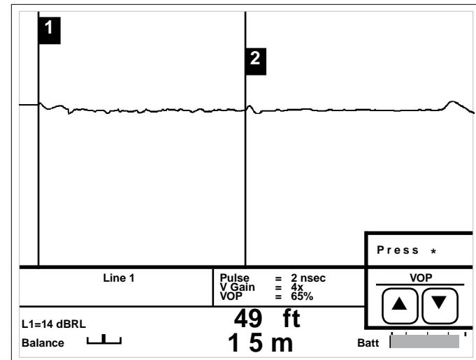
A telephone BUILD-OUT CAPACITOR causes a low impedance DOWNWARD reflection (similar to a SHORT) followed by a smaller positive reflection.
