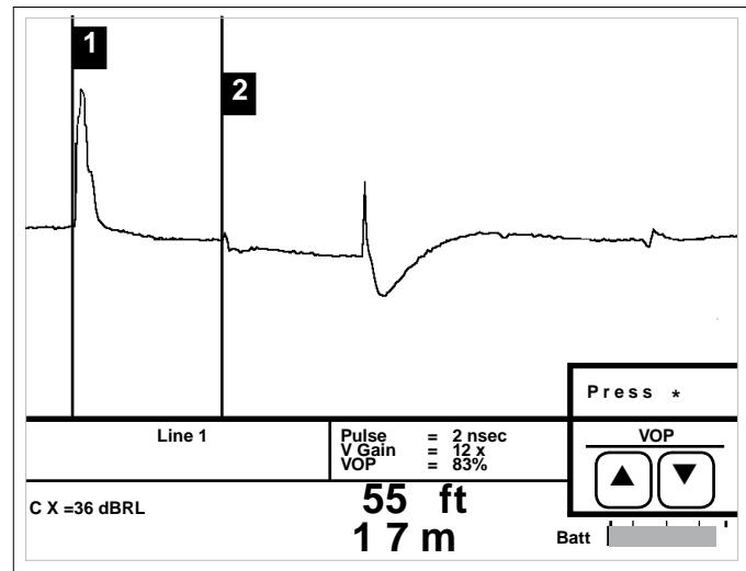
A splitter or directional coupler can be identified although accurate measurements are difficult due to multiple reflections. The 2nd cursor identifies the splitter. The two reflections following are the ends of each of the cable lengths.
