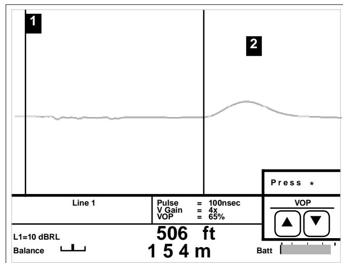
A reflection with upward polarity indicates a fault with OPEN (high impedance) tendencies. The reflection shown at the second cursor is a COMPLETE OPEN.
