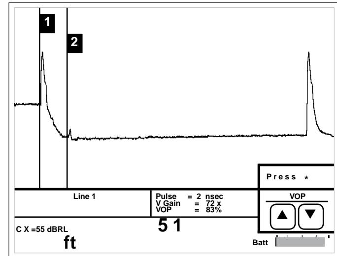
Due to attenuation, the reflections caused by each equally spaced taps are progressively smaller. A larger reflection (2nd cursor) beyond a smaller reflection may indicate an unterminated or faulty tap.
