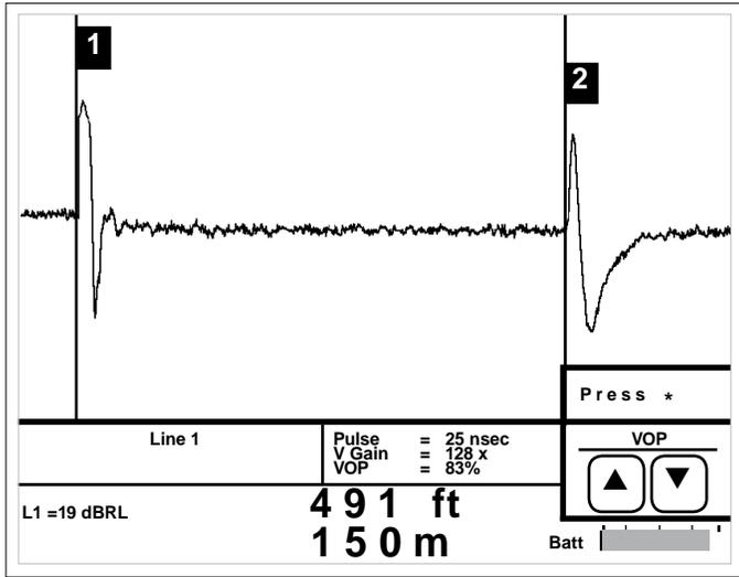
Testing tower cables with antennas can be challenging due to energy induction from high RF areas as shown in this waveform. Stepping through various noise filter settings will result in a “cleaner” waveform.
