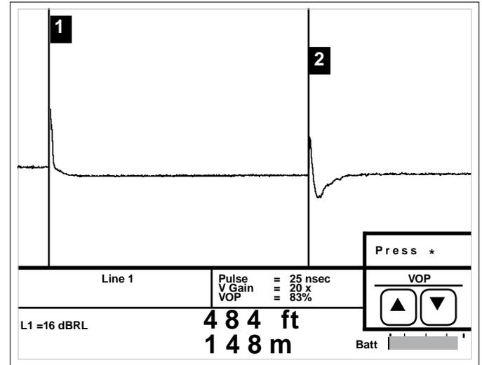
Testing through to an antenna usually results in a "S" shaped reflection, although reflections can vary greatly depending on the antenna.
