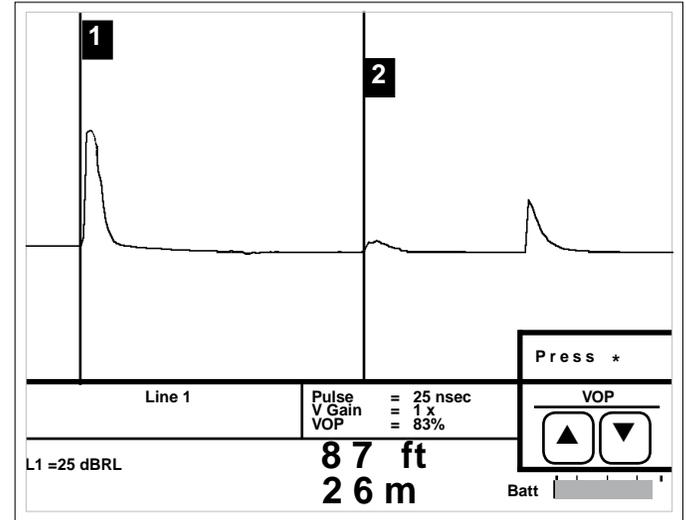
The middle reflection at the 2nd cursor is a partial open followed by a complete open (end of the cable). The more severe the fault, the larger the reflection.
