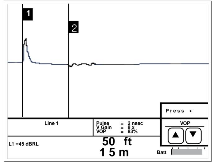
A water-soaked cable will display a waveform with a downward slope indicating the beginning of the water and an upward rise at the end of the water. Generally, the area between the two reflections will appear “noisy.”
