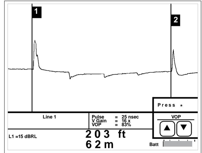
Coaxial taps (both indoor and outdoor) will cause reflections along the waveform. The quality and value of each tap determines the amount of reflection.
