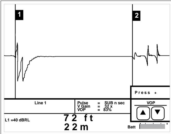
The three events seen in this section of 750 CATV hardline are a minor dent, a major dent, and a questionable splice.
