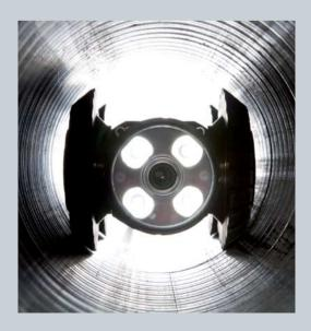
operate fully submersed and are water resistant to depths of up to 100m (330'). They are constructed from brass and stainless steel and are built with a single or twin 50W motor configuration, powerful enough to move through almost any pipeline system. The integrated sensitive inclinometer and the multi-frequency sonde allow you to map pipeline topography easily and efficiently.
