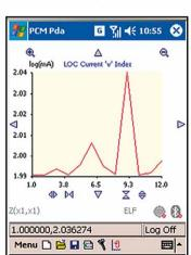
The Radiodetection Survey software incorporates GPS information and shows the mapped data in a variety of formats as well as allowing comparisons between new and old mapping surveys.
