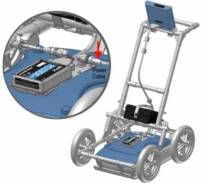
Figure 2.7: powering the sensor box
