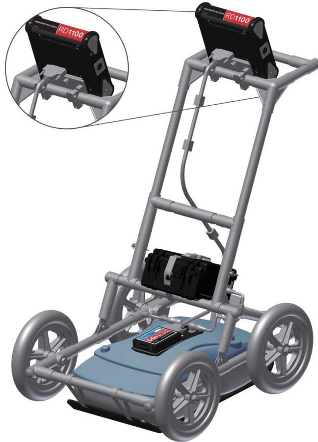
Attach the Odometer and Battery Cables. The Odometer Cable connects to the closest receptacle on the Sensor. Attach the Battery Cable to the Sensor and the Battery. The system is now set up and ready to use.
