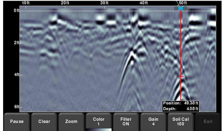
The menu at the bottom of the screen allows you to change viewing parameters, such as gain, filter, colour and zooming (for depth and horizontal position).
