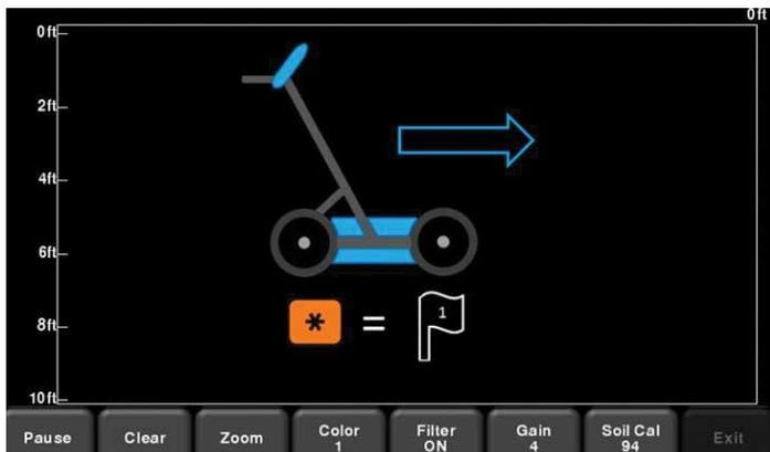
You are ready to start collecting data by simply pushing the system. The data scrolls from right to left.
