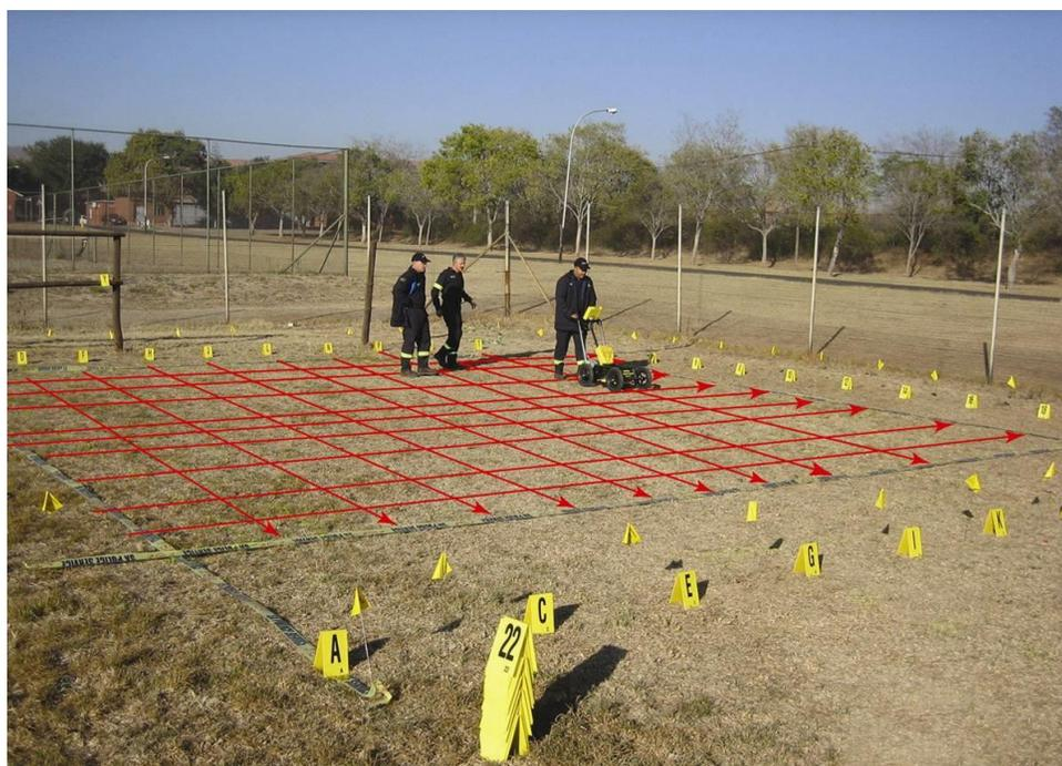
*Figure 9-3: Example of a grid survey. The red lines are superimposed just to illustrate the concept.*
