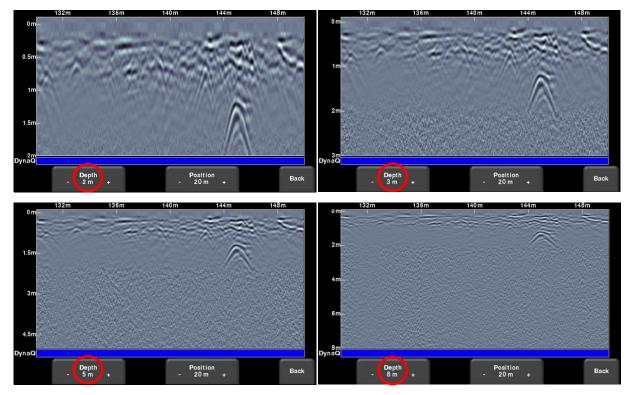
Figure 8-7: Varying displayed depth
