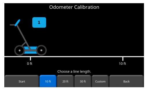
Figure 6-20: Odometer Calibration - select a distance and then press Start
