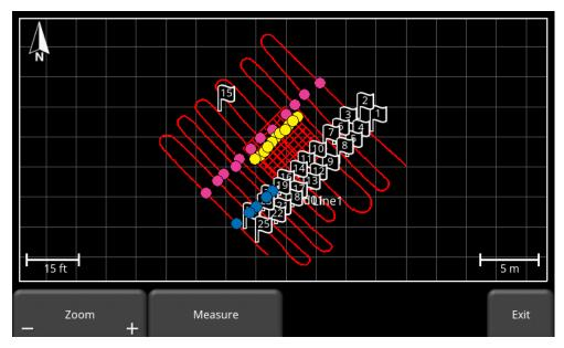
Figure 6-10: Map View showing two grids and a long line with interpretations. Map View is enabled because the data was collected with GPS.
