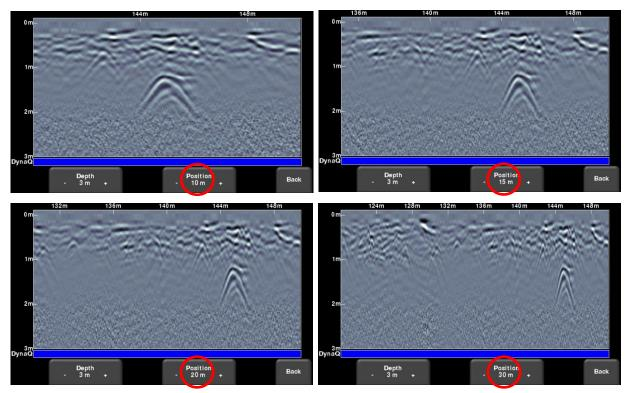
Figure 8-8: Varying position or horizontal scaling
