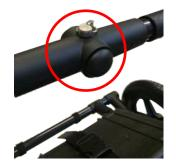
With the pole pointing upwards, insert the GPS mount into the opening where the plug was located, and secure it with the quick release pin. This allows the GPS to sit directly over the middle of the GPR sensor. It comes with 5/8-11 UNC-1A threads at the top of the pole, which is standard for many GPS receivers.
