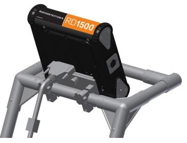
Connect the other end of the cable to the Sensor. Ensure the cable is routed as shown below.
