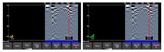
Figure 8-4: a) Back-up Indicator, b) Moving the Depth Indicator to the top of the hyperbola
