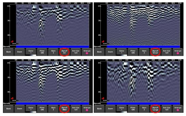
Figure 8-12: FrequenSee<sup>™</sup> settings: a) Top left shows **All**. b) Top right set to **Small** targets. c) Bottom left set to **Medium** targets. d) Bottom right set to **Large** targets
