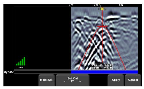
Figure 8-13: Adjusting Soil Cal while in backup mode
