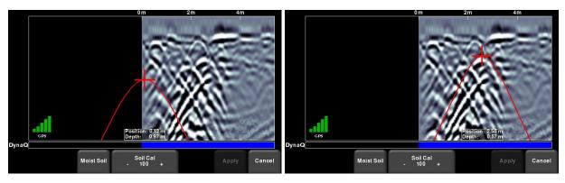
Figure 8-14: Adjusting Soil Cal, without backing up
