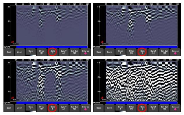
Figure 8-11: Varying the Gain
