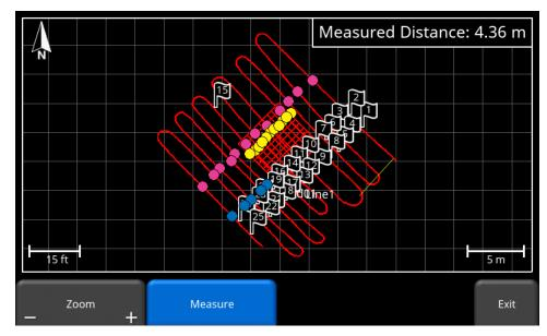
Figure 11-4: Using the Measure tool to draw a line on the screen
