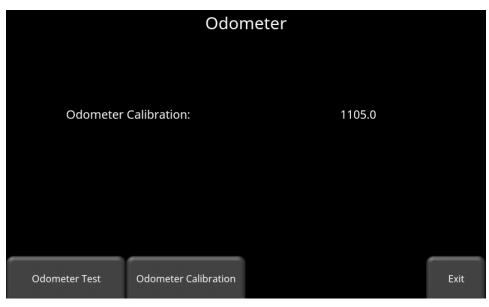
Figure 6-17: Screen displaying current odometer calibration
