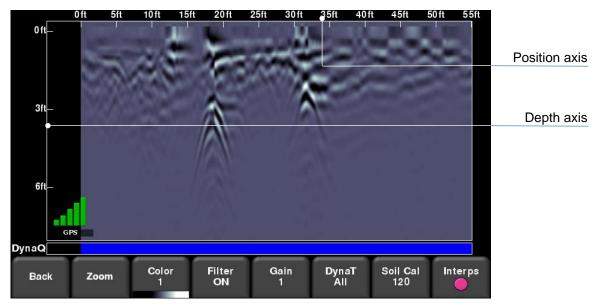
Figure 8-3: Line Scan acquisition mode, showing collected data and axis labels
