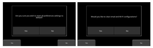
Figure 6-7: Reset to Defaults, a) Image on left is the first confirmation screen. b) If you press **Yes**, you will see the second confirmation screen on the right asking about deleting e-mails and WiFi settings.
