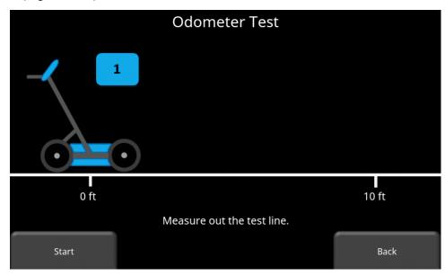
Figure 6-18: Doing an odometer test
