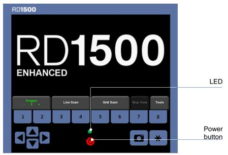
Figure 5-1: Front of Display Unit
