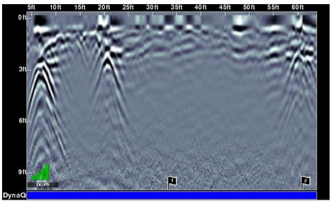
Figure 8-6: Inserting Flags
