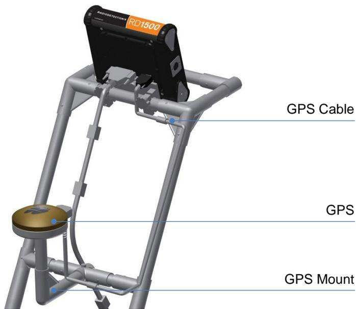
GPS – If you have purchased the Topcon GPS from Radiodetection, this can be screwed onto the threads at the top of the GPS mount. Connect one end of the GPS cable to the GPS receiver, and the other end to the serial port on the back of the Display Unit. This single cable powers the GPS and receives data from it.
