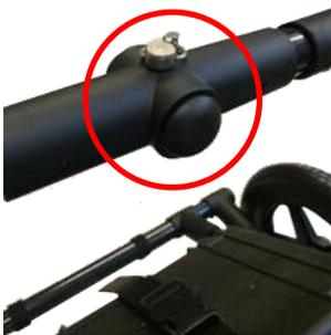
With the pole pointing upwards, insert the GPS mount into the opening where the plug was located, and secure it with the quick release pin. This allows the GPS to sit directly over the middle of the GPR sensor. It comes with 5/8-11 UNC-1A threads at the top of the pole, which is standard for many GPS receivers.
