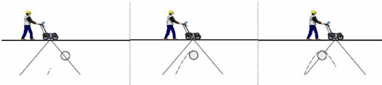
Hyperbolas are best viewed when subsurface targets are crossed perpendicularly or at a 90 degree angle. The actual position of the object is located at the apex of the hyperbola.
