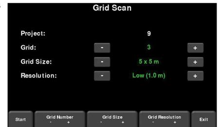
Align the system so that the longitudinal axis is centered on the first line. Then line up the middle of the sensor with the starting line and press **Start**. Push the system in a straight line towards the end of the line. Data acquisition will automatically stop once you reach the end of the line. The Line Scan image of the data just collected will appear on the left side of the screen.
