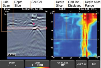
Pressing the + and - buttons on the Depth button will increase or decrease the depth of the depth slice currently displayed. This allows the user to "slice through" the ground, and locate features that appear at different depths.
