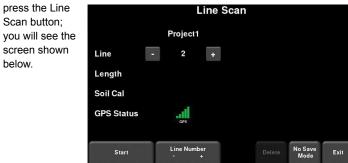
Press the Start button to begin collecting data. The screen will change to the data acquisition screen. As the system is pushed along a straight line, the collected GPR data scrolls onto the screen from the right and moves to the left
