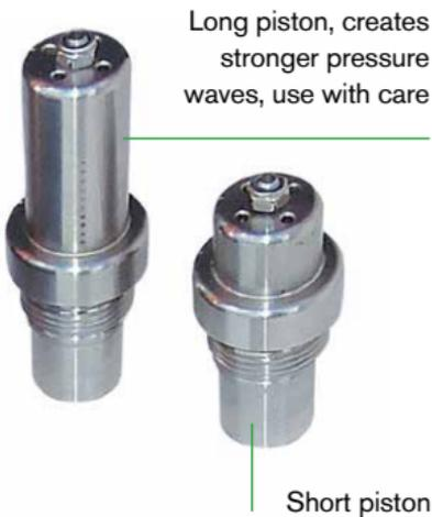
It is possible to vary the strength of the pressure wave created by the RD550 using the different pistons provided. The larger piston creates a stronger pressure wave. As stronger pressure waves put the pipe infrastructure under greater stress we recommend starting with the shorter piston.
