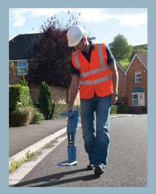
STRIKEALERT Alerts the operator to the presence of shallow power cables.
