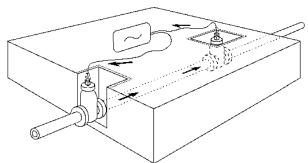
Figure 7.5: Making double-ended connections
