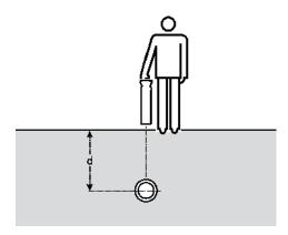
Figure 6.1: Taking a depth reading
