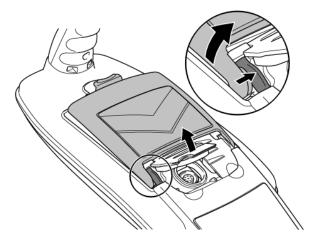
Figure 4.4 Press the retaining latch inwards
