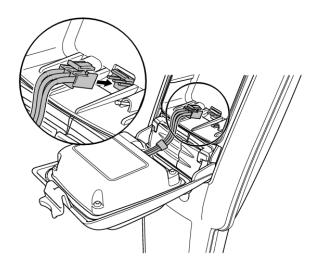
Figure 4.7 Connecting the Li Ion lead
