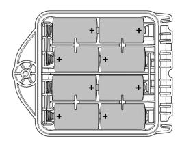
Figure 4.3 D-cell battery trays
