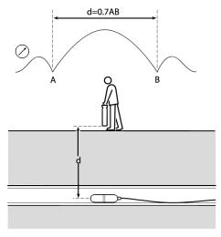
Figure 8.10: Calculating sonde depth
