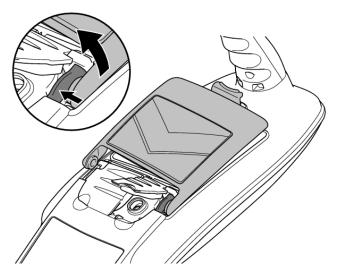
Figure 4.5 Repeat then lift the battery pack away
