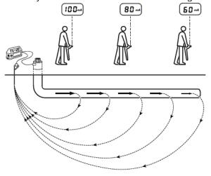
Figure 6.7: Current readings using transmitter signals
