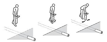
Figure 5.2: Pinpointing a target line
