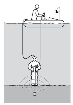
Figure 8.12: Using a submersible antenna
