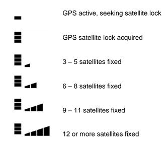
Figure 4.15 GPS status and satellites in view
