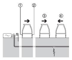
Figure 9.1: Cable sheath fault-finding
