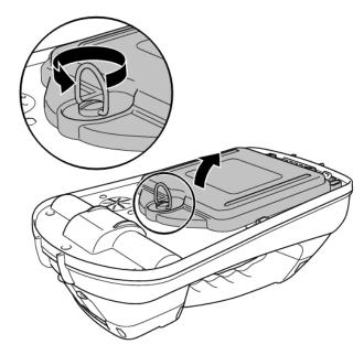
Figure 4.9: Opening the battery compartment
