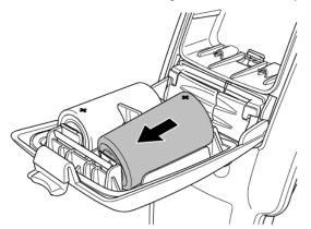
Figure 4.2 Inserting locator batteries
