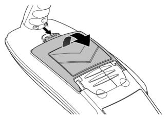
Figure 4.1 Open the battery compartment
