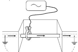
Figures 8.5 – 8.6: Connecting transmitter clamps
