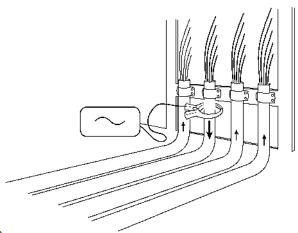
WARNING!. The transmitter must only be connected to live services using the appropriate accessory such as a plug connector or live cable connector.
