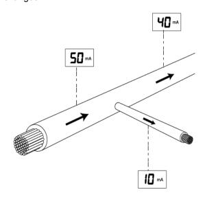
Figure 6.3 Current readings
