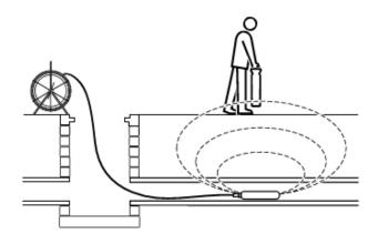
Figure 8.8 Sonde deployment
