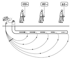
Figure 6.7: Current readings using transmitter signals
