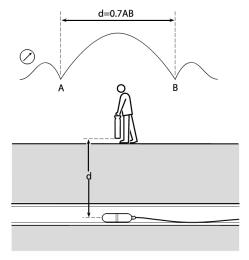
Figure 8.9: Calculating sonde depth
