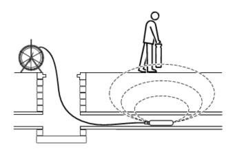
Figure 8.7 Sonde deployment
