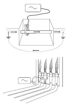
Figures 8.4 – 8.5: Connecting transmitter clamps
