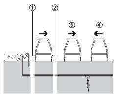
Figure 9.1: Cable sheath fault-finding
