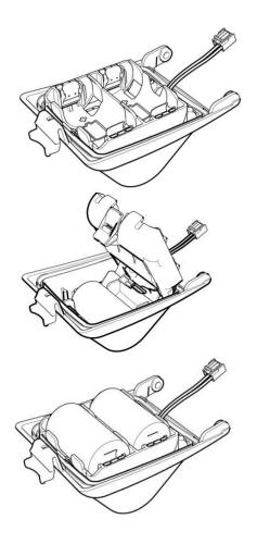
Figure 3.4 Locator D-cell holder
