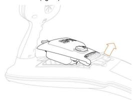
Figure 3.7 Rotating the battery pack
