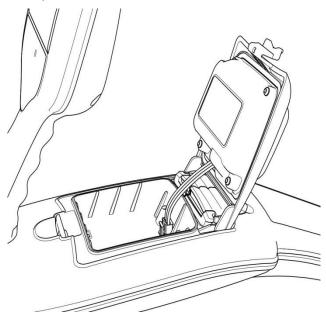
Figure 3.1 Li-ion battery pack connection
