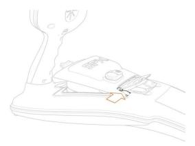
Figure 3.6 Pressing retaining latch
