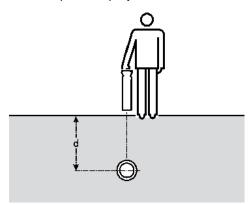
Figure 6.1: Taking a depth reading
