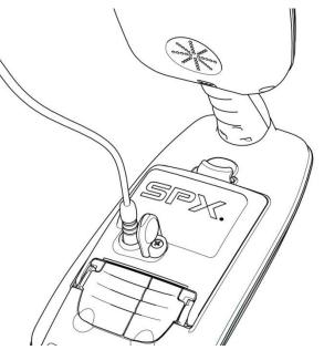
Figure 3.2 Charging the locator Li-ion battery pack
