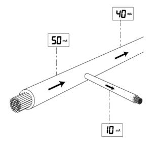
Figure 6.3 Current readings
