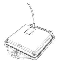
Figure 3.3 Charging the transmitter Li-ion battery pack
