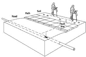
Figure 9.2: Locating faults with the locator and A-frame
