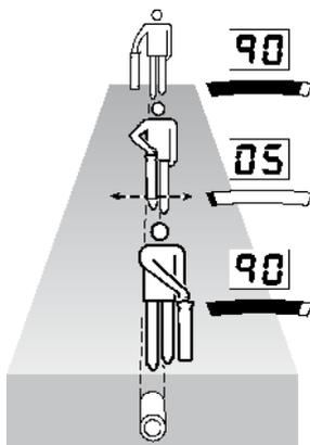
Figure 4.1: Line Tracing
