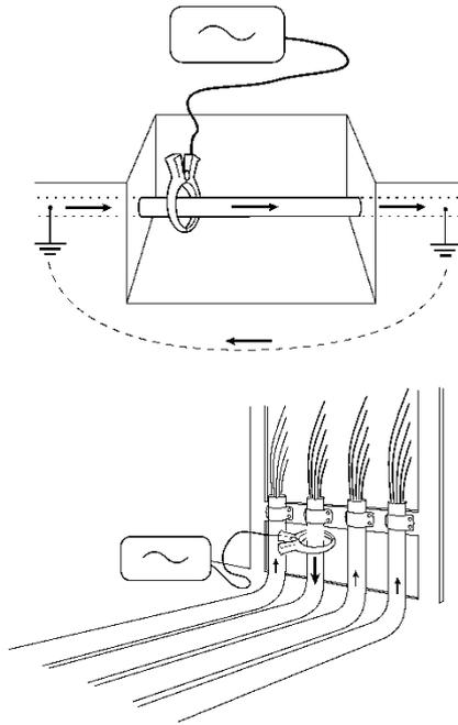
Figures 8.4 – 8.5: Connecting transmitter clamps
