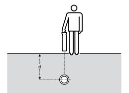
To avoid signal distortion, do not apply the signal by induction. If direct connection or signal clamping is not possible, place the transmitter at least 15m (49ft) from the point of any depth measurements.
