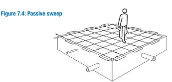
Stop when the locator response rises to indicate the presence of a line. Pinpoint the line and mark its position. Trace the line out of the area being searched. Resume grid search in the area.
