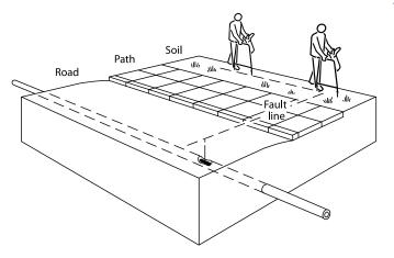
Take readings at the survey intervals determined by the reference reading. To locate the cable during a Fault-Find survey, press the (a) key once and the locator will switch to 8kHz null mode. Locate the cable using the normal null mode technique. Press the (a) key again to return to Fault-Find mode.
