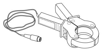
WARNING!. The transmitter must only be connected to live services using the appropriate accessory such as a plug connector or live cable connector.
