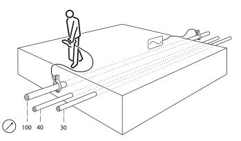
To ensure that the target cable has been correctly identified, reverse the positions of the transmitter and locator and check that the strongest response is still received from the target cable by the locator in its new position.
