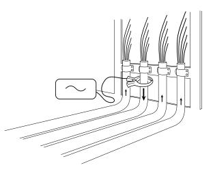
NOTE: It is not necessary to make a ground connection from the transmitter when using the clamp.
