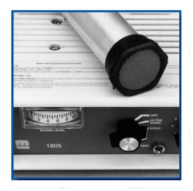
The Dielectric Model 1805 Multisonic Detector pinpoints leaks in pressurized cable systems by converting both sonic and ultrasonic sounds into visual and audible signals. Designed to span the range of frequencies from 100 Hz to 100 KHz, the Model 1805 quickly detects both large and small pressure leaks. Unique circuitry enhances leak sounds while diminishing unwanted background noises. A sensitive meter responds to low signal levels cueing the user to listen for difficult to detect leaks.
