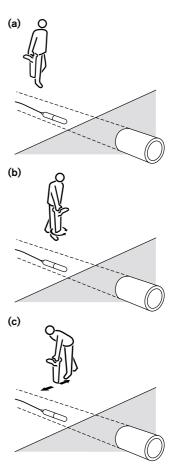
Propel the sonde a further three to four paces along the drain or duct and pinpoint and mark. Repeat this procedure along the route at similar intervals. It should only be necessary to change the locator sensitivity while tracing the sonde if there is a change in the depth of the drain or duct, or the distance between locator and sonde.
