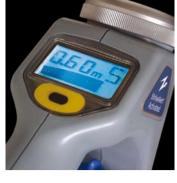
In Sonde/CPS Mode deployed sonde frequencies or Cathodic Protection Systems (CPS) are detected.
