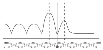
Just prior to the fault, the signal will rise dramatically and then fall to a null followed by a slightly smaller peak. The fault will lie at the null point between the peaks. The 'lay effect' should be virtually zero past the fault.
