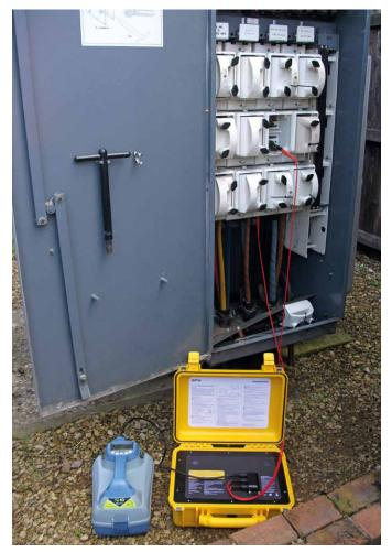
Select a frequency between 512Hz / 640Hz and 1kHz and set the desired output power. Generally an indicated locate frequency current of over 100mA will be required to ensure a clear cable lay effect.
