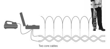
The rise and fall of the response should be regular and with a pronounced null between each peak (although the sharpness of the null will become less distinct as the signal is traced further along the cable due to stray signal pick-up on the other cores or the sheath).
