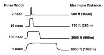
Sometimes, larger pulse widths are helpful even for locating faults that are relatively close. If the fault is very small, the signal strength of a small pulse may not be enough to travel down the cable, "see" the fault, and travel back. The attenuation of the cable combined with the small reflection of a partial fault can make it difficult to detect. A larger pulse width would transmit more energy down the cable, making it easier to see a small fault.
