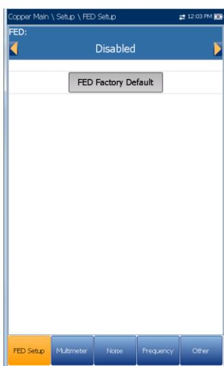
When **FED** is **Auto** or **Manual** and you start a test, the 6100-Cu will warn you if the FED battery level is low. Select **OK** to close the message and run the test. Also, if the FED is not present or not responding, a **Confirmation** dialogue box will be displayed asking if you want to disable FED and run the test anyway.
