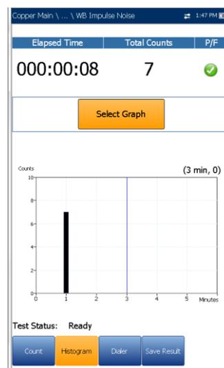
**Select Graph** button changes to **Graph Selected** when pressed and opens a new selection of function keys which allow you to maneuver the graph as follows:
