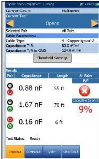
The **Snapshot** page shows measured **Capacitance** values and **Length** for each lead combination. The parameters are as follows:
