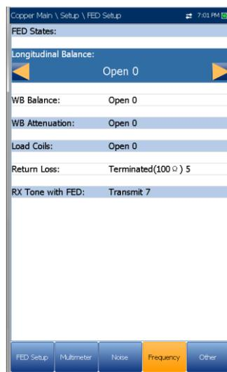
Default values are displayed for **WB Attenuation**, **RX Tone with FED**, and **Load Coils**.
