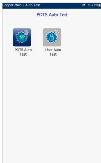
**Auto Test** allows you to automatically run tests used in pre-qualification, installation, and maintenance of different circuit types from POTS to VDSL2. The main menu allows you to select and run the displayed tests:
