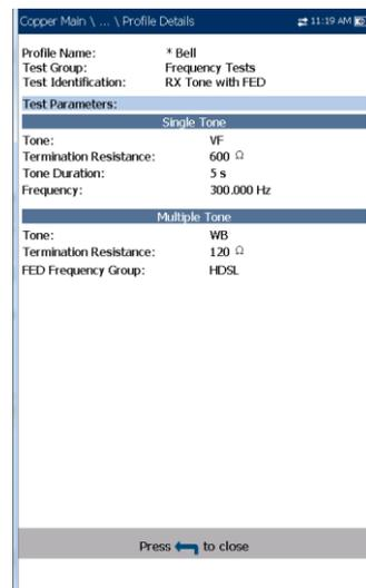
The **Profile Details** page displays read-only **Test Parameters** for both the Single and Multiple RX Tone with FED tests, and may contain the following entries:
