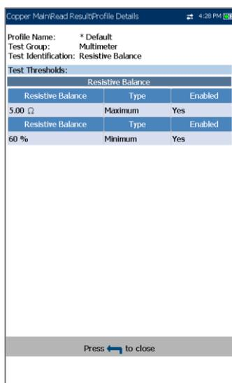
The **Profile Details** page displays read-only **Resistive Balance** thresholds.
