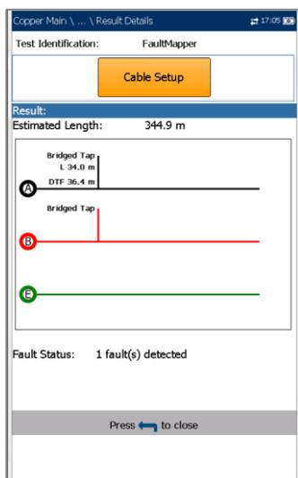
The **Result Details** read-only page displays the test results in text and graphical format.
