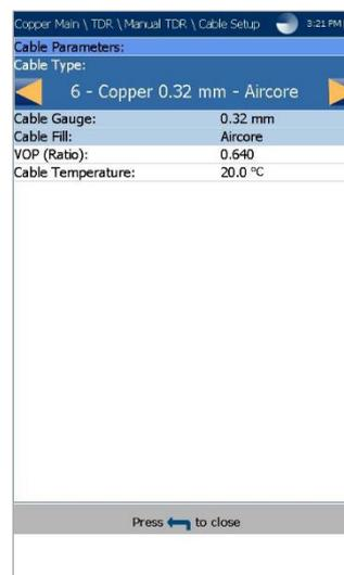
The **Cable Setup** page allows you to configure and/or view the **Cable Parameters** set for the TDR test.
