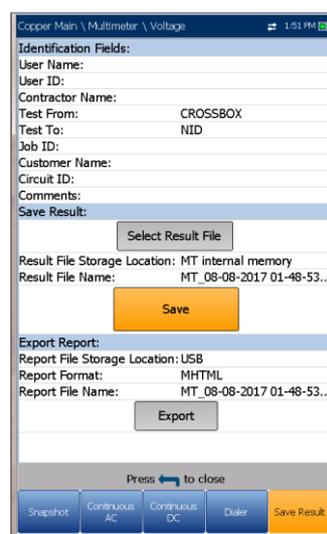
Alternatively, when a test is completed or stopped and you press
