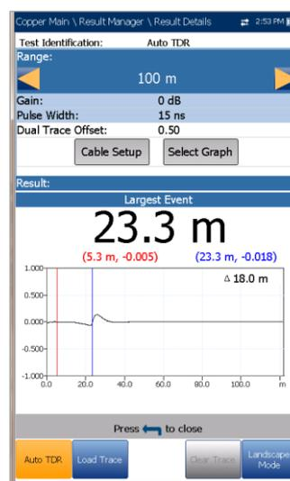
Results are shown in text and graphical format in **Portrait/Landscape Mode**. You can load a saved auto TDR trace (secondary trace) and display it simultaneously with the original TDR trace (primary trace).
