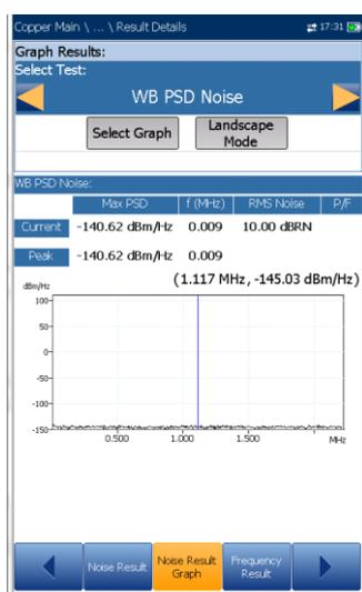
The **Noise Result Graph** page displays the pass/fail status and results in graphical format for the following noise tests:
