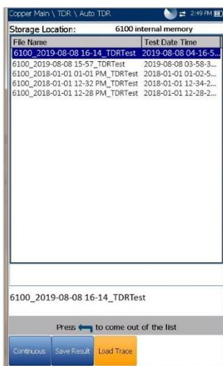
The **Load Trace** function allows you to load a saved trace. The tab opens a page listing previously saved TDR tests by **File Name** and when the test was saved, that can be used as the trace files to be loaded. A trace may be loaded:
