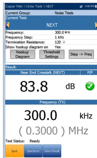
**Spot** is a continuous mode of operation measuring the crosstalk for a specific frequency selected by you, similar to the method used by the **Send Tone** test. The **Spot** function displays and updates results in real time, until you stop the test. The last valid results then remain displayed.
