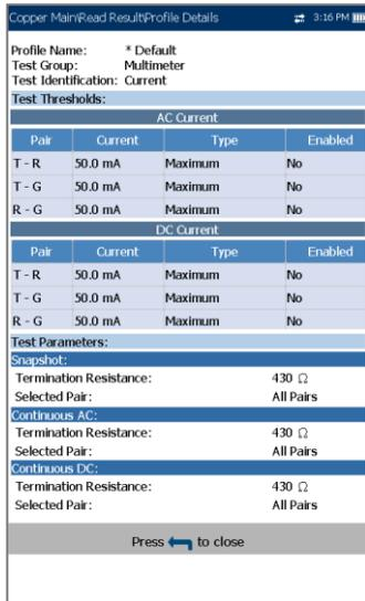
The **Profile Details** page displays read-only test thresholds and/or parameters information about the setup of the selected test, and may contain the following entries:
