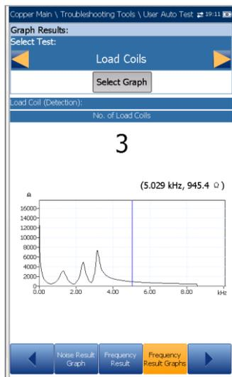
The **Frequency Result Graphs** page displays the results in text and graphical format for the following frequency tests:
