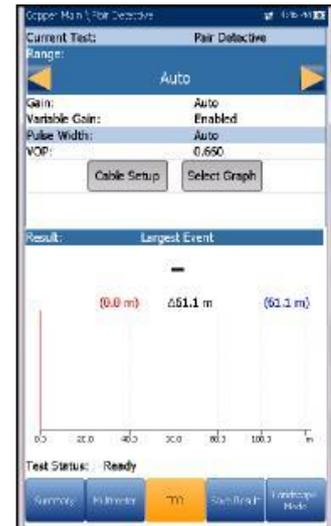
The **TDR** test displays the line trace and is continuously on and ready to use. It displays and updates results in real time, in either **Portrait** or **Landscape Mode** (recommended), until you stop the test. The last valid results then remain displayed.
