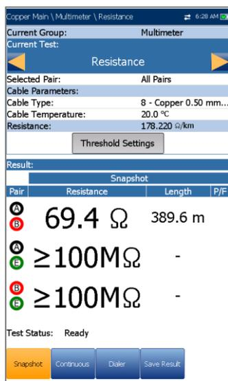
The resistance **Snapshot** shows measured resistance values in Ohms and cable lengths for each lead combination. The parameters are as follows:
