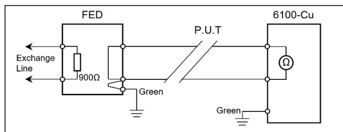
*Note: P.U.T., in the above diagrams, refers to the Pair Under Test.*
