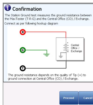
The hookup diagram uses the following graphic and textual components:
