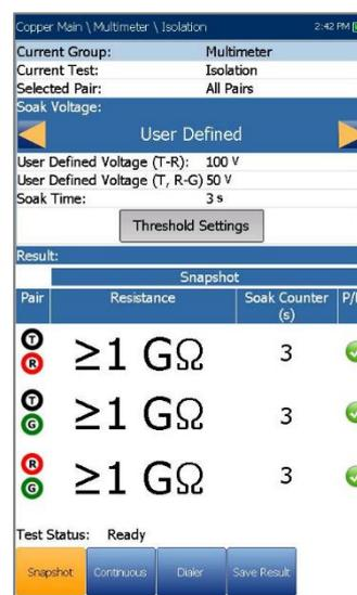
The **Snapshot** page shows measured isolation resistance values for each lead combination. The parameters are as follows:
