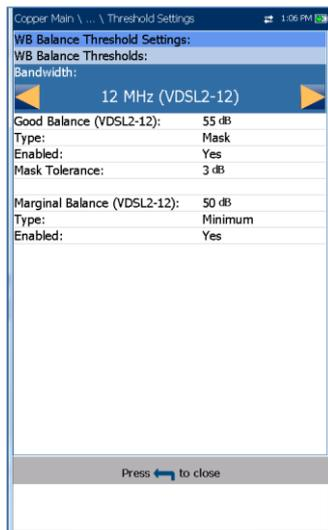
The **Threshold Settings** page allows you to set the **Good/Marginal Balance** thresholds for the following:
