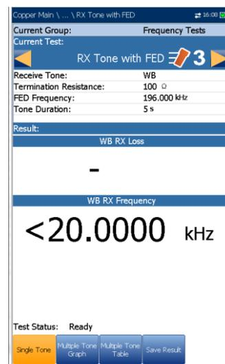
The **Single Tone** tab allows you to configure the following parameters:
