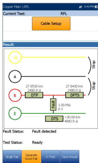
Connect a strap from the faulted wire to both conductors of the good pair.
