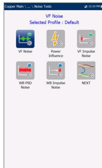
The **Noise Tests** menu allows you to select and run the displayed tests:
