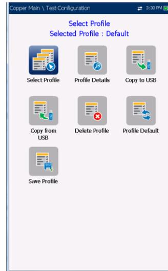
The **Test Configuration** menu provides the utilities to setup test parameters. The 6100-Cu supports several types of copper test applications. Test parameters and thresholds are saved into a test configuration profile. A Profile Default is provided with a predefined set of parameters for all test applications.
