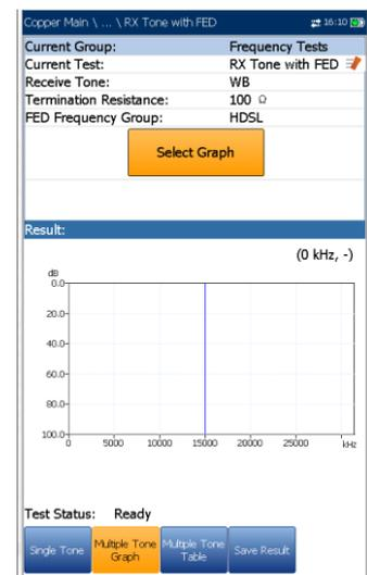
The **Multiple Tone Graph** tab displays results in text and graphical formats. From this page, you can run the **RX Tone with FED** test using multiple frequencies, by configuring the following parameters:
