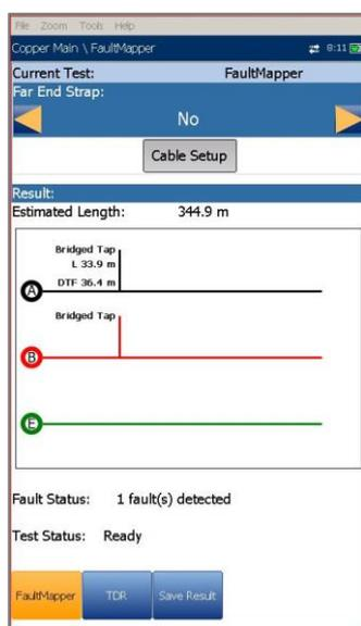
The **FaultMapper** page displays the following parameters:
