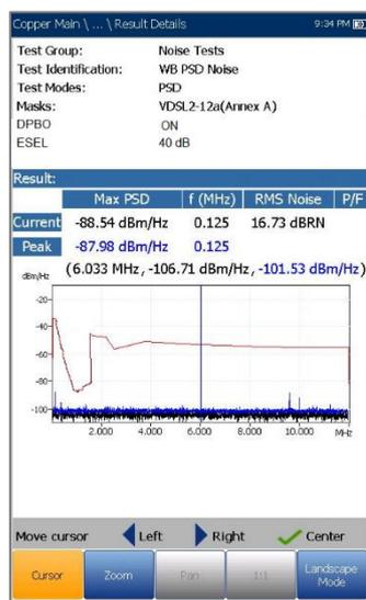
The **Results Details** read-only page displays the WB PSD Noise test results, in text and graphical format. If an ESEL (Exchange Side Electrical Length) value was set, it is also displayed. The graph can be viewed in portrait and landscape modes, and maneuvered as follows:
