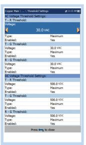
**Thresholds** are customised for Pass/Fail test indications, including:
