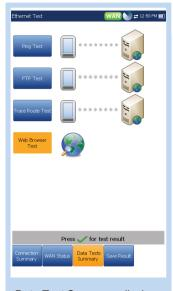
**Data Test Summary** displays the pass/fail status of the selected data tests enabled in the connection setup including:
