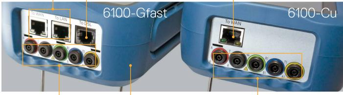
Banana connectors supporting G.fast/DSL and copper testing
