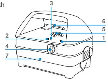
Genny4 signals can be detected by all previous 33 kHz C.A.T models including C.A.T<sup>3</sup>. C.A.T4 will also locate Genny<sup>3</sup> signals.
