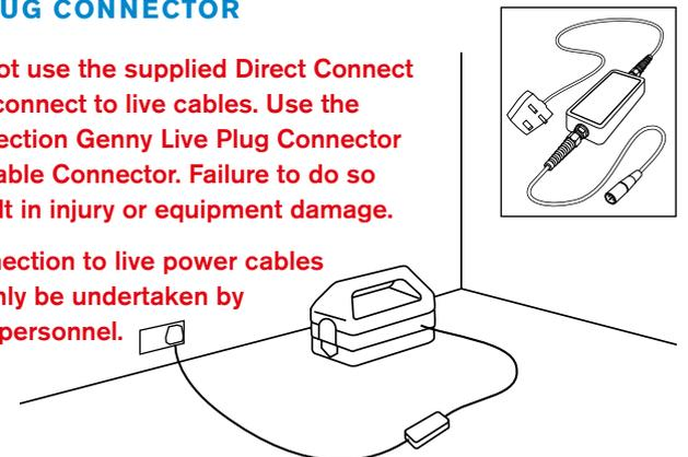
The Live Plug Connector applies the Genny signal to a live domestic power socket and, via the domestic wiring system, to the service and supply cable in the street.
