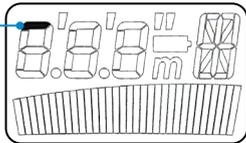
**NOTE: When a valid depth measurement is displayed, the GPS icon will momentarily disappear from the screen.**
