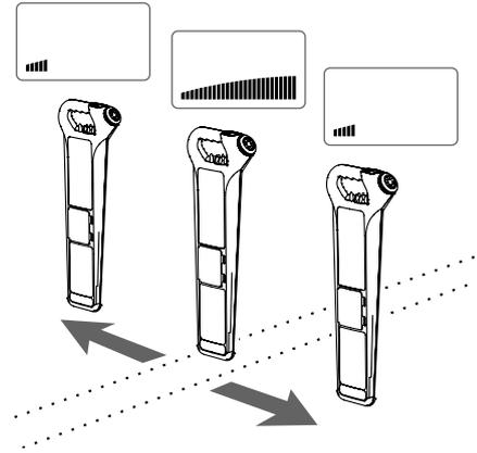
If the position cannot be easily determined using Avoidance Mode, switch between the dedicated locate modes (Genny, Power or Radio) before adjusting the sensitivity control to pinpoint the cable or pipe.
