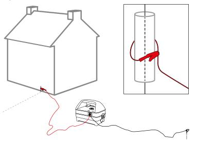
Signal jumping from an accessible cable
