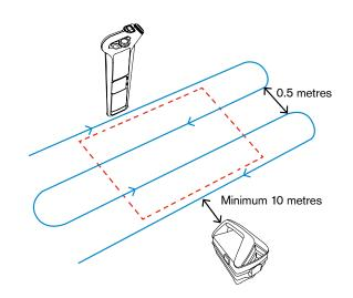
Active search using Induction – finding parallel pipes and cables
