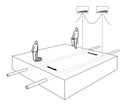
Eliminating adjacent cables or pipes ('Nulling out')
