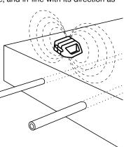
Estimating line depth using the C.A.T4+/gC.A.T4+ and Genny4
