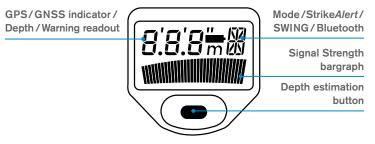
NOTE: The screen in gC.A.T4 models may remain active for up to 30 min, depending on the locator's settings. Refer to the GPS/GNSS Operation paragraph for further info.
