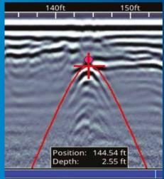
Use hyperbola-fitting to ensure accurate depth measurements and backup over the target to display its location and depth.
