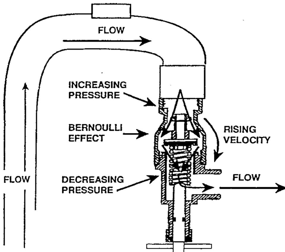
Larger diameter pipes require higher flow rates to produce a strong signal output. The three types of Pulse Transmitters currently offered are summarized in Table 2.1 below:
