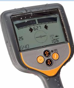
Built for on-site use – IP65 Shock resistant, ingress protected casing protects against knocks, drops, water and dust.
