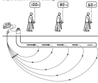
Figure 6.7 - Current readings using transmitter signals
