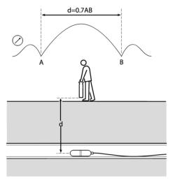
Figure 8.6 - Calculating sonde depth
