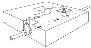
Figure 7.5 - Making double-ended connections
