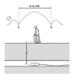
Figure 5.5 - Verifying a depth measurement
