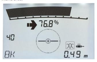
Figure 5.4 - Depth readings
