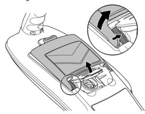
Figure 4.3: Press the retaining latch inwards
