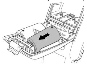
Figure 4.2: Inserting locator batteries
