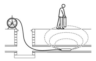
Figure 5.1 Sonde deployment
