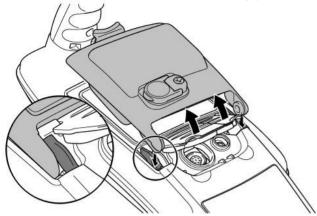
Figure 4.5: Installing a new battery pack
