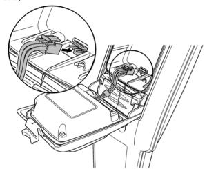
Figure 4.6: Connecting the Li Ion lead
