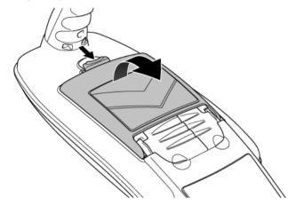
Figure 4.1: Open the battery compartment
