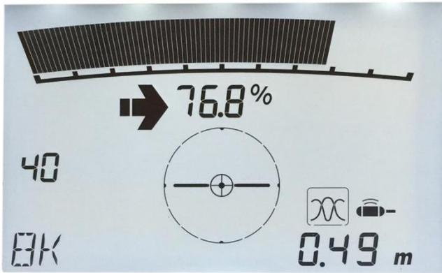
Figure 5.4 – Depth readings
