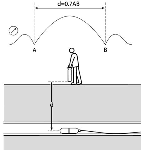
Figure 5.5 - Verifying a depth measurement
