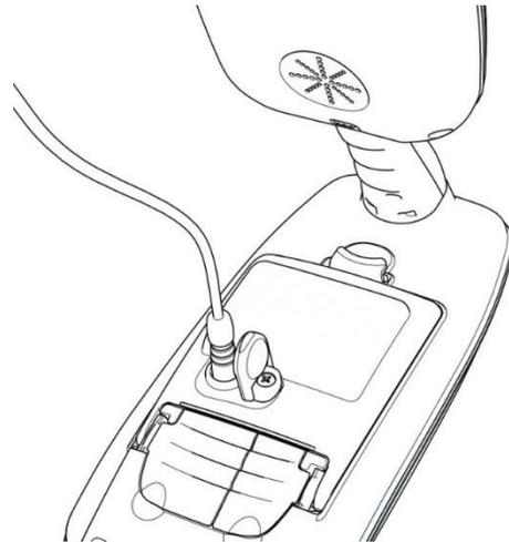
Figure 4.7 - Charging the locator Li-ion battery pack
