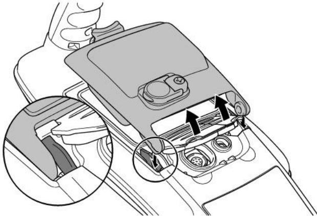
Figure 4.5: Installing a new battery pack
