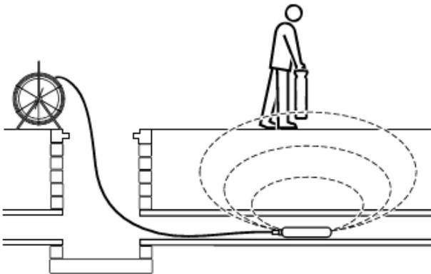
Figure 5.1 Sonda deployment
