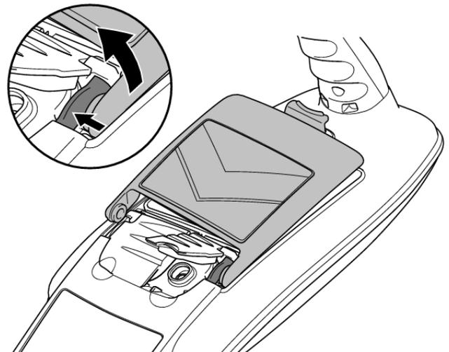
Figure 4.4: Repeat then lift the battery pack away
