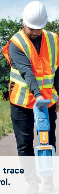
Using a transmitter is essential to identify and trace buried utilities, as it puts the operator in control.
