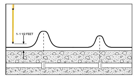
Figure 17: Signal Patterns Provided by Cast-Iron Pipes
