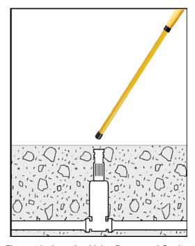
Figure 16: Locating Valve Boxes and Casings
