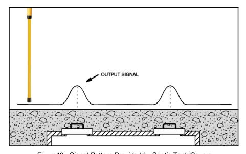
Figure 12: Signal Pattern Provided by Septic Tank Covers
