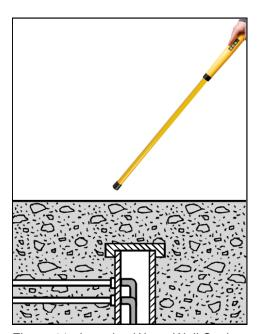
Figure 11: Locating Water Well Casings
