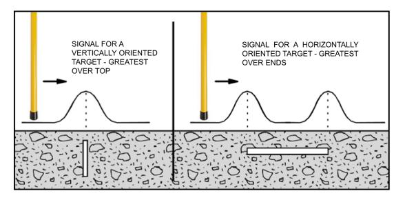
Figure 5: Signals from Vertical and Horizontal Targets
