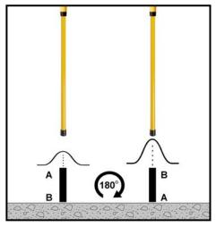
Figure 9: Checking a Stake's Orientation
