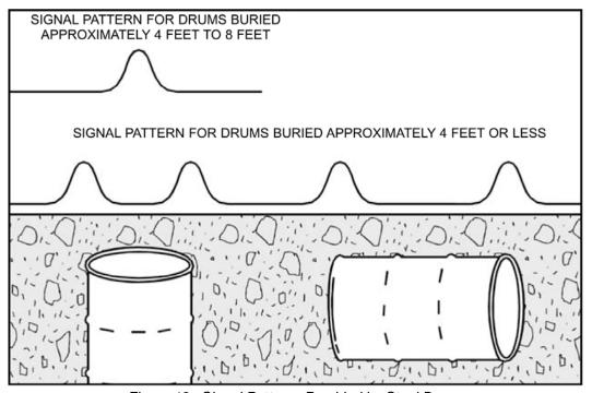
Figure 18: Signal Patterns Provided by Steel Drums
