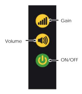
Figure 2: SPOT® Membrane Switch
