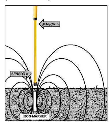
Figure 1: Detecting the Magnetic Field of an Iron Marker
