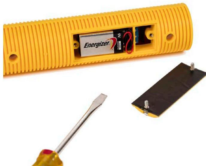
Figure 3: Replacing the Battery
