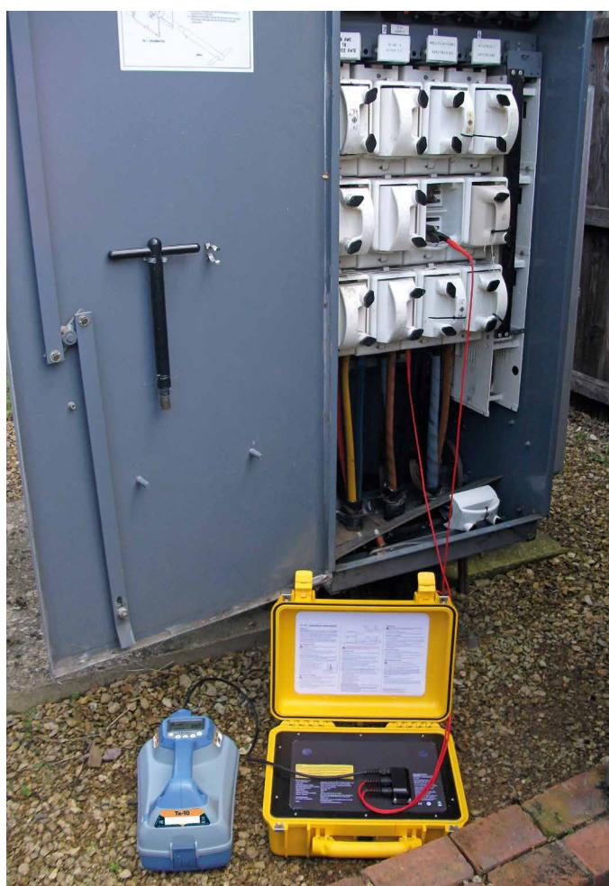
Select a frequency between 512Hz / 640Hz and 1kHz and set the desired output power. Generally an indicated locate frequency current of over 100mA will be required to ensure a clear cable lay effect.
