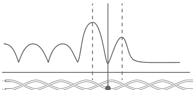
Just prior to the fault, the signal will rise dramatically and then fall to a null followed by a slightly smaller peak. The fault will lie at the null point between the peaks. The 'lay effect' should be virtually zero past the fault.
