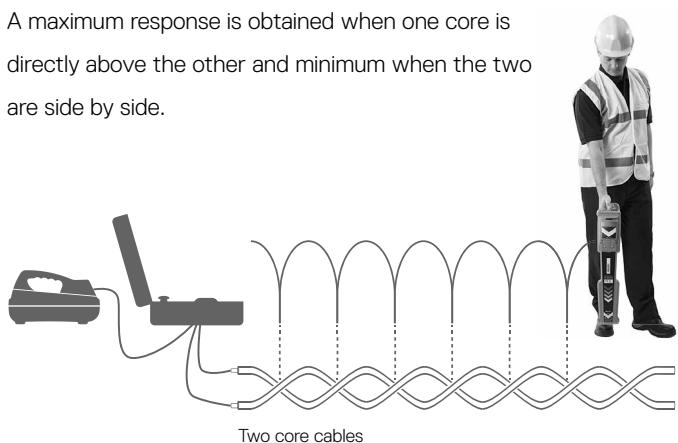
The rise and fall of the response should be regular and with a pronounced null between each peak (although the sharpness of the null will become less distinct as the signal is traced further along the cable due to stray signal pick-up on the other cores or the sheath).
